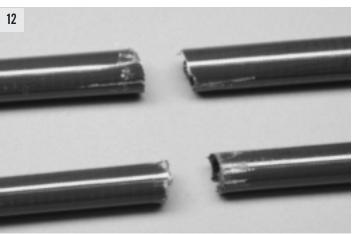
you no longer have a tube and a catastrophic failure is the result. Load limit failures are easy to spot. This type of break will always take place in the bottom half of the rod, usually just forward of the handle or the fisherman's furtherest point of effort (the rod hand). The break will be slightly irregular with jagged edges and short lengthwise splits and tears (9). Looking at the inside of an overload failure you'll note great distress in the walls of the blank both inside and out (10).
